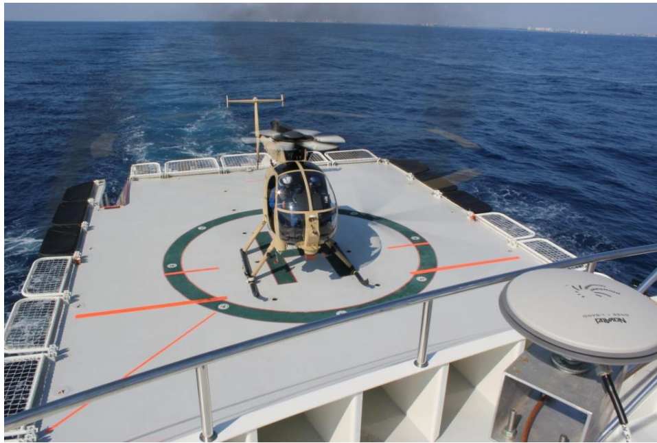
Figure 12. Safe landing zone visual cues (orange lines)
