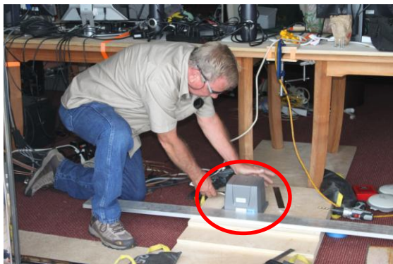
Figure 19. SPAN IMU installation
