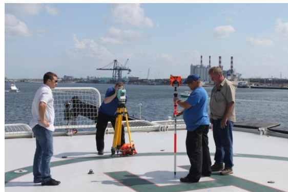
Figure 20. Total station survey
